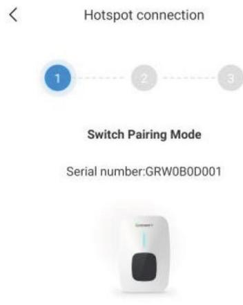
Before switching the hotspot mode, please make sure that the EV Charger is not connected to the network cable
